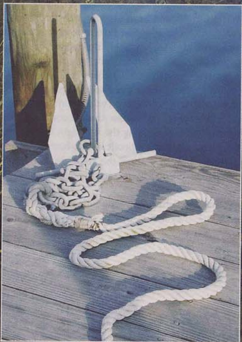
This angler found it easier to slip an anchor over than to stake out his push-pole. Left, a small fluke-style anchor and plastic-coated chain is ideal, and will also hold in deeper water.
