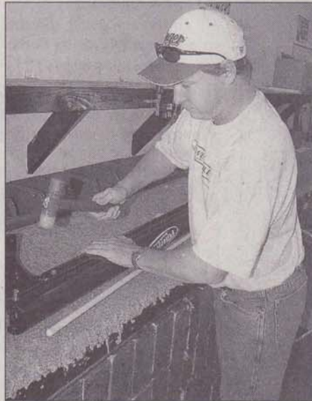
Plant manager Bob Shamblin taps home an assembly pin on a Power-Pole.
